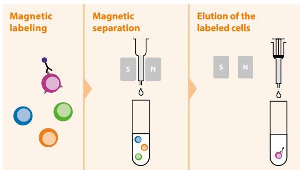
**Figure 4: Positive selection with MACS Technology.** Target cells are magnetically labeled. During separation, the magnetically labeled cells are retained within the column, while unlabeled cells flow through. After a washing step, the column is removed from the magnetic field of the separator and target cells are eluted from the column.
